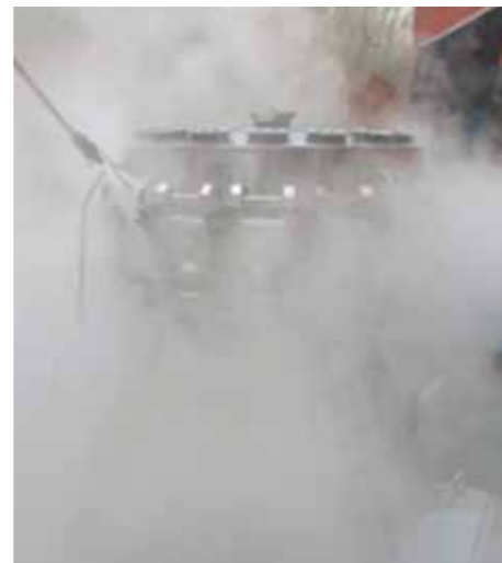
Under-going high pressure jetting test for IPX9k
